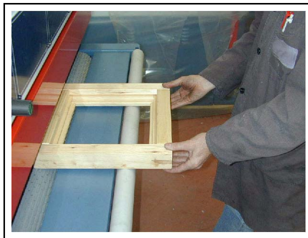
Fig. 2.2 Correct workpiece grip
